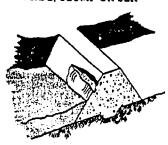
Earth or rocks move down the slope along a slippage surface because of too steep a slope, or the foundation moves. Also, look for slides movement in reservoir basin. **HAZARDOUS**
