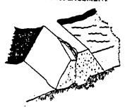
1. Vertical movement between adjacent sections of the ambankment.
