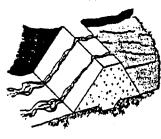
1. Severe drying has caused shrinkage of embankment material.
