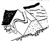
Excessive travel by livestock especially harmful to slope when wet.
