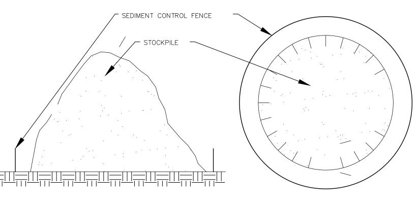
SEDIMENT CONTROL FENCE TO BE INSTALLED AROUND STOCKPILE (SEE SEDIMENT CONTROL FENCE DETAIL).
